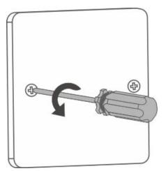
(2) Align the mounting holes of the bracket with the screw holes in the 86 mm junction box. Then, secure the bracket to the junction box using Phillips pan head screws (M4 x 20 mm).
