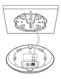
b Align the slots on the rear of the AP with the square feet on the mounting bracket, and slide the AP into the mounting bracket slowly to ensure that the AP is secured.
