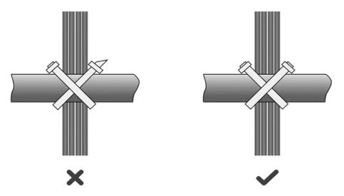
• When cables need to be bent, bind them first, but do not tie cable ties within the bend. Otherwise, stress may be generated on the cables and causes the wires inside to break, as shown in Figure 7-5.
