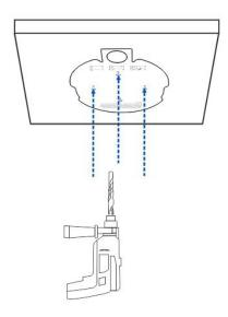
(2) Secure the mounting bracket to the ceiling or wall using wall anchors and Phillips pan head screws (M4 x 20 mm).
