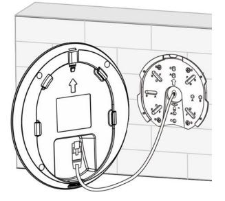
(4) Align the slots on the rear of the AP with the square feet on the mounting bracket, and slide the AP into the mounting bracket slowly to ensure that the AP is secured.
