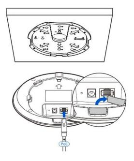
b Align the slots on the rear of the AP with the square feet on the mounting bracket, and slide the AP into the mounting bracket slowly to ensure that the AP is secured.
